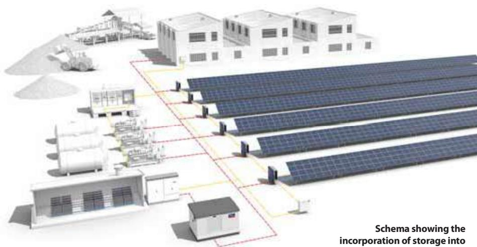
Schema showing the incorporation of storage into a PV-diesel hybrid system.
