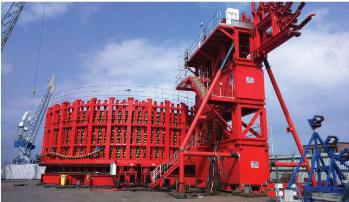
Dutch subsea cable installer, Blue Offshore, fashioned a unique “double basket” carousel barge to move 8,000 tons of cables from the manufacturing site in Greece to Rotterdam
